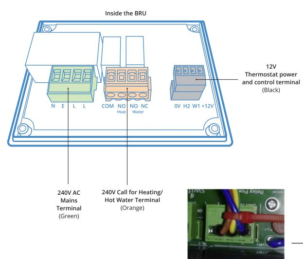
**Important:** If the current boiler control operates at a low voltage, connect the appropriate low voltage to the COM (common) and do not add the jumper cable.
